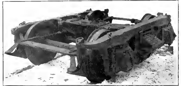
Truck Which Combines Passenger and Freight Features
